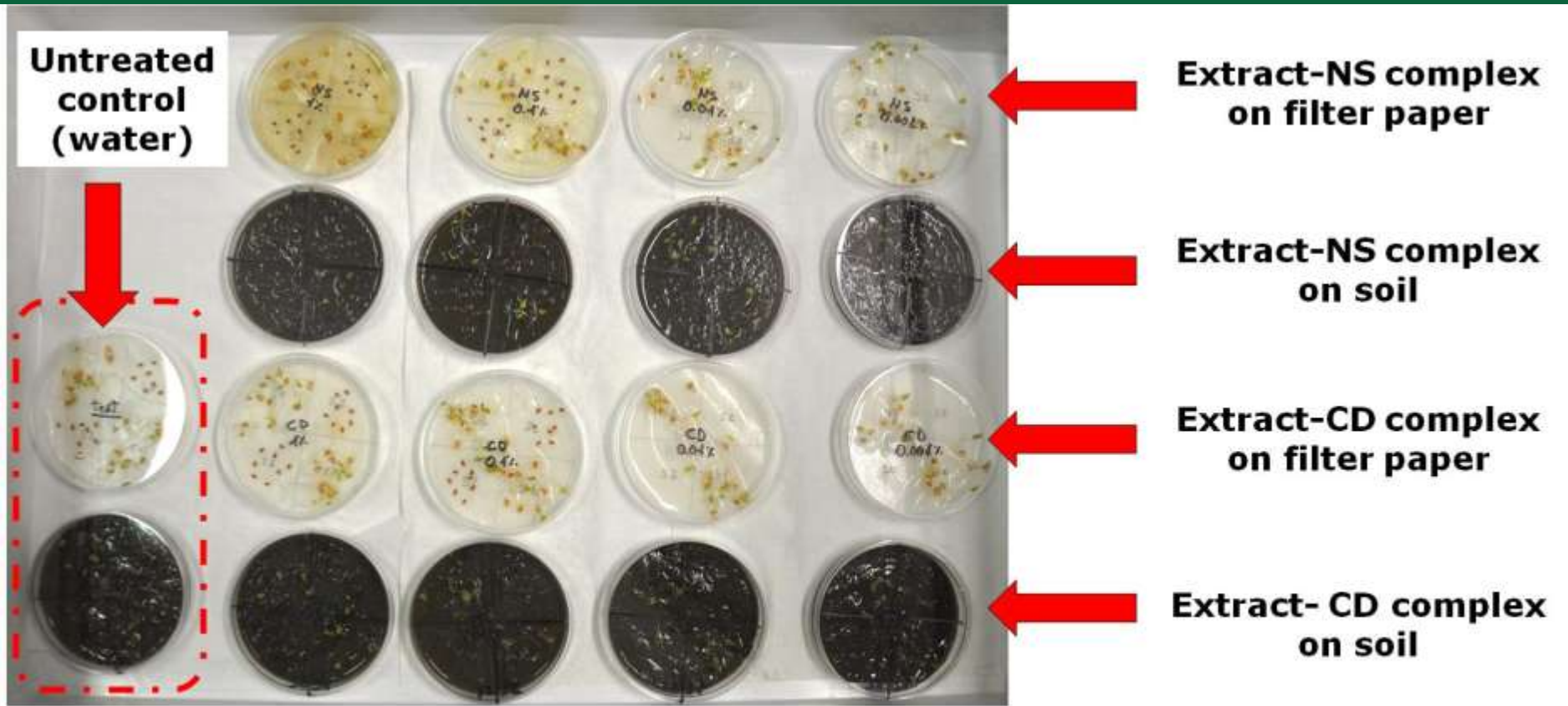
Germination test: Lepidium seeds treated with the extract of A. altissima included in \beta -cyclodextrins (extract-CD complex) or in \beta -cyclodextrin based nanosponges (extract-NS complex), at different concentrations (ppm): 5000, 500 , 50, 5.
